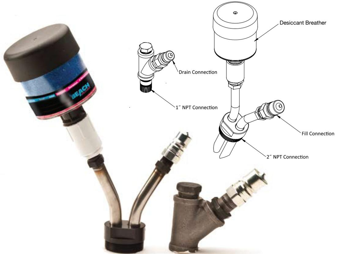
Beach tote adapter kits incorporate quick connect fittings and desiccant breather filters to function as the connection between your application and filtration system. Pairing fluid handling filtration with breather protection allows for maximum system integrity—requiring less equipment and labor while reducing system contamination.
