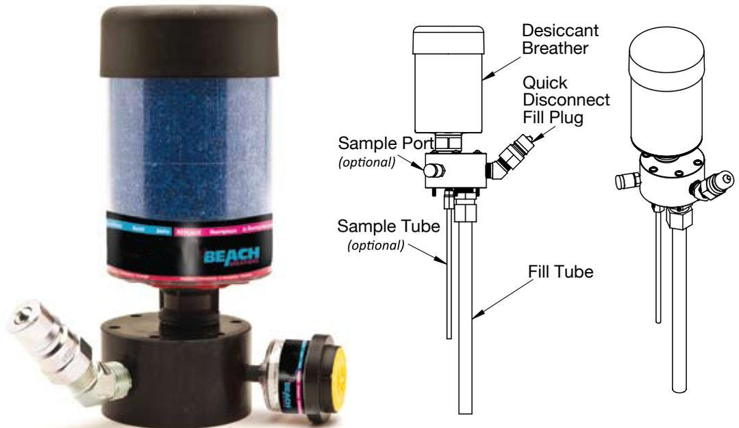
Beach hydraulic adapter kits incorporate quick connect fittings, desiccant breather filters, vacuum indicators, and sample ports to function as the connection between your application and filtration system. Pairing fluid handling filtration with breather protection allows for maximum system integrity – requiring less equipment and labor while reducing system contamination.
