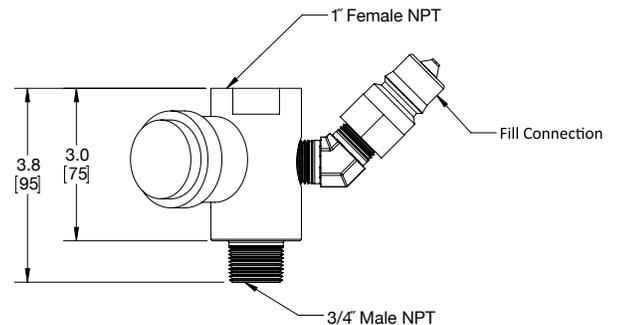
Beach gearbox adapter kits incorporate quick connect fittings, desiccant breather filters and vacuum indicators to function as the connection between your application and filtration system. Pairing fluid handling filtration with breather protection allows for maximum system integrity—requiring less equipment and labor while reducing system contamination.
