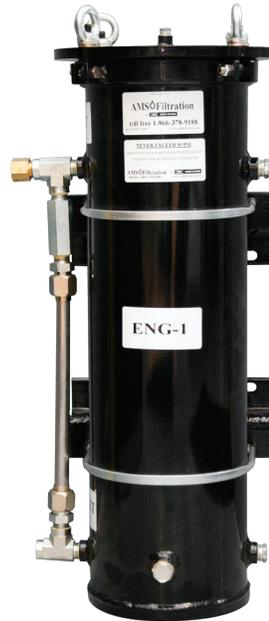
Contaminated oil results in excess machine wear, downtime, and repair costs. Actively filtering lubricants can prevent contamination-related problems.
