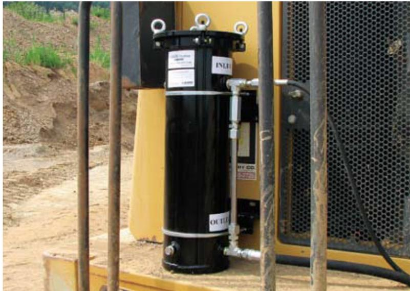
Contaminated oil results in excess machine wear, downtime, and repair costs. Actively filtering lubricants can prevent contamination-related problems.
