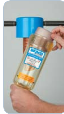
Remove bowl and dirty scrubber. Clean scrubber thoroughly with warm water and soap only.
