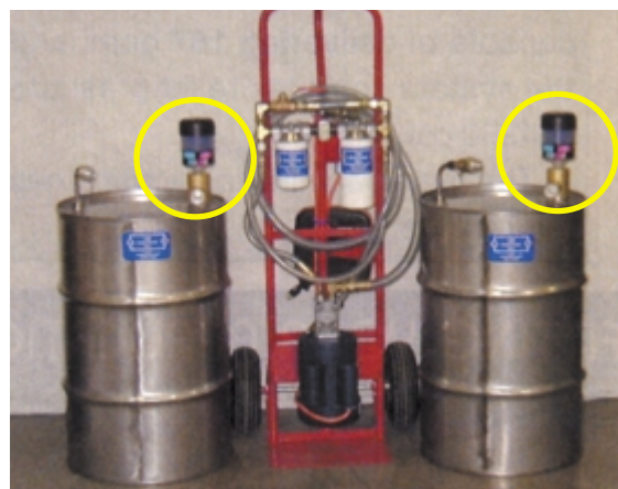
The air breather (circled in yellow on each drum) uses a desiccant to remove moisture from any air vented into the drum when the fluid level lowers.
