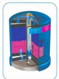
Beach is now carrying a new disposable steel breather for outdoor and marine applications. This rugged breather is designed for big cylinder systems like garbage trucks and construction equipment. The BB/DS-6 is 6.5" tall x 5" in diameter with a filtration area of 38 in and a 9 oz, absorption capacity, its operating temperature range is -20°F to +250°F. Look for more information about this new product soon.
