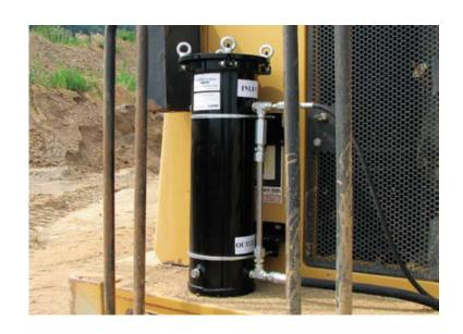
Contaminated oil and hydraulic fluid result in excess machine wear, downtime, and repair costs. Actively filtering lubricants can prevent contamination-related problems.
